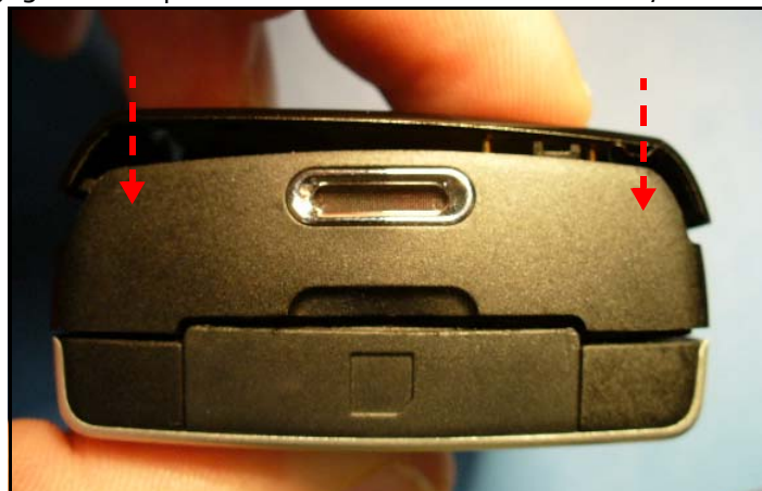
Figure 3: E-cover assembly installation
