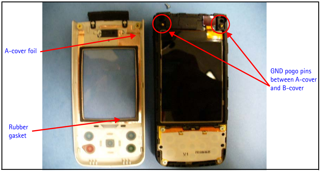
Figure 24: A-cover foil and GND pogo pins
