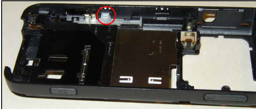
Figure 13: BT antenna inner catch inside D-cover
